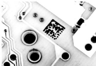
Figure 33 - Data Matrix Code Directly Marked on PCB Surface by Using Laser Etching Technology
