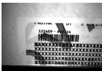
Figure 26 - Overprinted Barcode Readable also Through the Envelope Window Film
