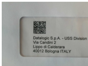
Figure 24 - Address Coded in Data Matrix Symbology for Automated Mail Processing
